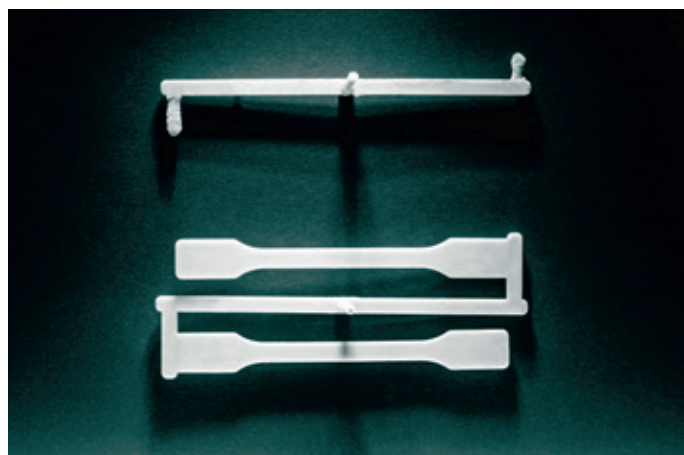
Figure 3: Grade of specimen-filling of PHAs — exemplarily PHBV — at the same injection moulding parameters (160 °C, 800/700 bar injection/holding pressure) without (at the top) and with 7 % of the polymeric additive bFI A 3745 (at the bottom).
